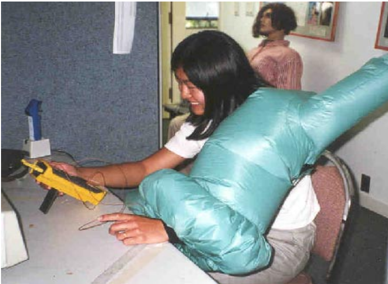
Figure 7: Temperature Controlled Air Sleeve for the Arm
