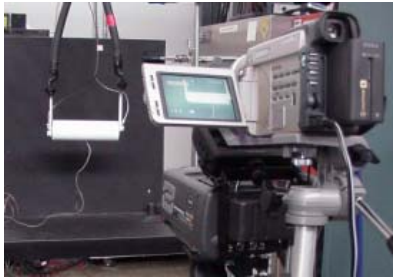
Thermal Imaging of a Saft Cell under 100 Amp Discharge
